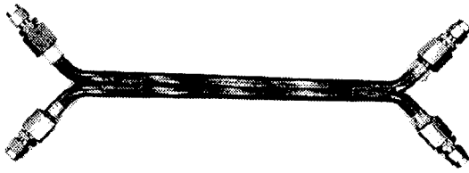
Fig.1. Nonuniform-line (linear-tapered) directional couplers with sliced coaxial cable.
